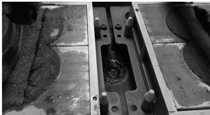
Figure 5 - Example of Excessive Fines in the Water Bath
