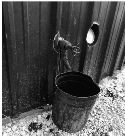
Figure 1 Examples of Valves Commonly Used for Sampling Liquid Asphalt from Tanks
